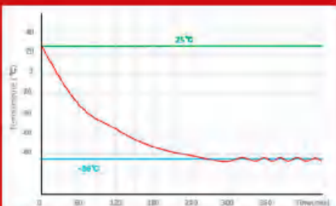
Pull down test at ambient temp. 25°C
