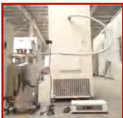
LN 2 /CO 2 backup system
